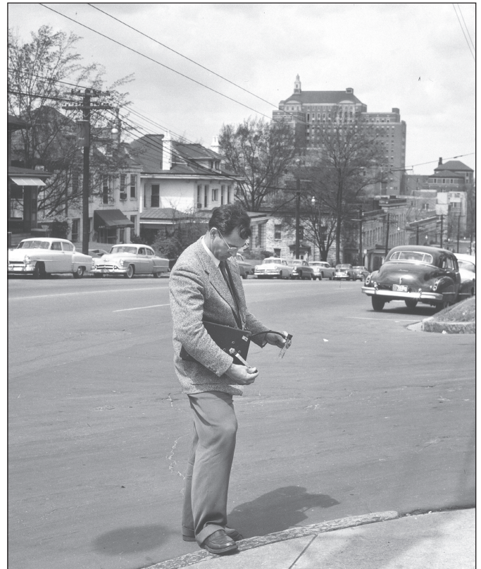
Collecting an Air Sample on 20th Street on Southside. Photograph by Bob Mitchell Studio, 1955. Courtesy Southern Research. Air pollution work at Southern Research during the 1950s included a program to collect, count, and measure dust particles in air samples taken in industrial and business areas.
